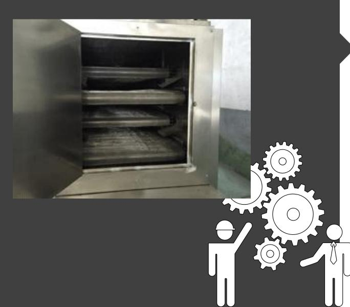
Drying machine is the cost-effective, and gets favorite responds from the buyers. Adjustable temperature makes Belt dryer have the capacity to dry more raw materials. After drying processing, the water content can reach to 10% or less. But the quality of raw material isn't damaged.
