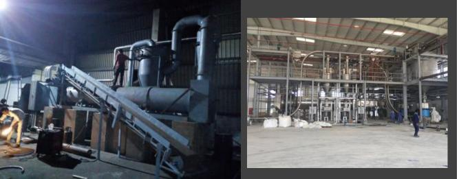
The rotary dryer is a type of industrial dryer employed to reduce or minimize the liquid moisture content of the material it is handling by bringing it into direct contact with a heated gas.
