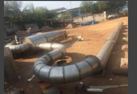
The principle of a flash dryer is simple. hot air (180oC) is sucked and mixed with the Wet product inside a very long pipe (called the flash pipe.The Wet product is passing through the pipe very quickly (in a "flash") and is dried to about 10% moisture.
